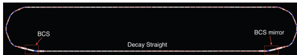
Figure 6: Racetrack ring layout. Pions are injected into the ring at the Beam Combination Section (BCS). Similarly, extraction of pions and muons at the end of the production straight is done using a mirror image of the BCS.
