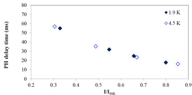
Fig. 6. Outer layer PH delays in coil 20 at 4.5 K and 1.9 K.
