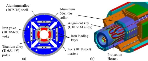
Fig. 1. (a)-HQ cross-section. (b)- Exploded view of the HQ02 magnet
