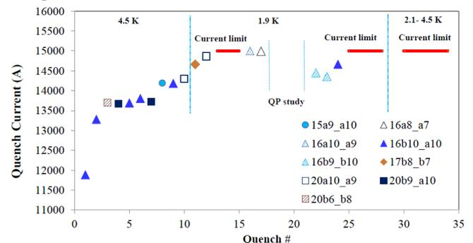
Fig. 3. HQ02 quench training at 4.5 K and 1.9 K. Voltage tap segments of the quench origin are also shown.
