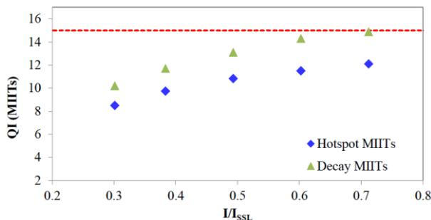
Fig. 8. QI as a function of the quench current ratio to the SSL at 1.9 K.
