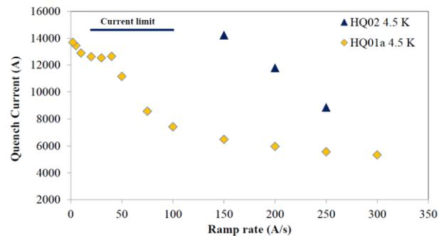
Fig. 11. Ramp rate dependence of the quench current in HQ01a and HQ02.
