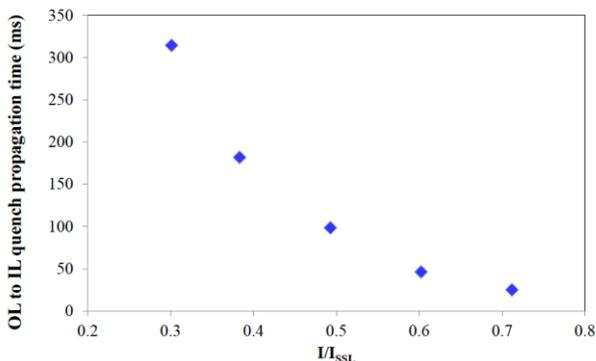
Fig. 10. Quench propagation time between the outer and the inner coil layers at 1.9 K
