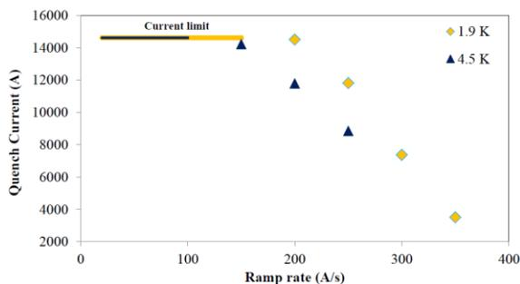
Fig. 4. HQ02 ramp rate dependence. Horizontal lines indicate the area of ramp rates without quenching up to the maximum quench current.
