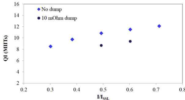
Fig. 9. QI without and with the extraction dump at 1.9 K.
