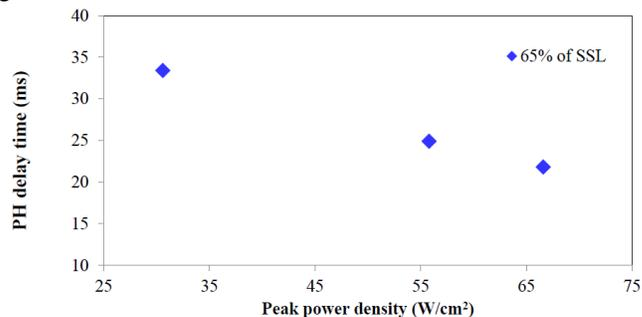
Fig. 7. Outer layer PH delay as a function of the peak power density measured at 1.9 K.
