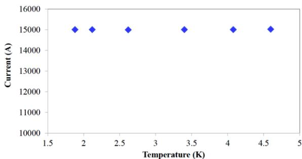
Fig. 5. Temperature dependence of the maximum current reached at a regular ramp rate of 20 A/s.
