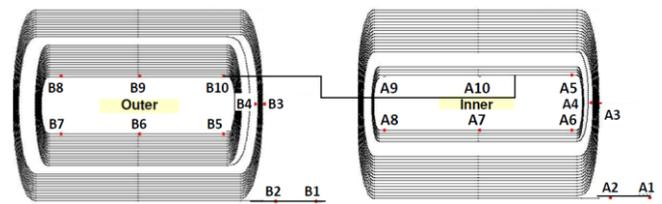
Fig. 2. Voltage tap location for the inner and outer coil layers.
