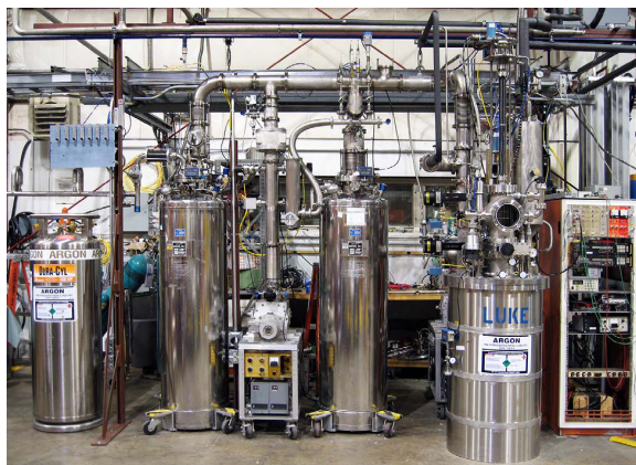
Figure 1. Photograph of the materials test system (MTS) at FNAL. Commercial argon (left) is passed through two filters (center) before entering the cryostat (right).
