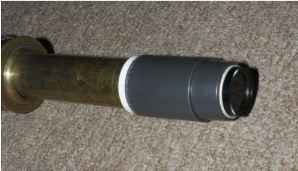
Figure V: Variable density (Moon) filter adapter used with refractor #1-AK.
