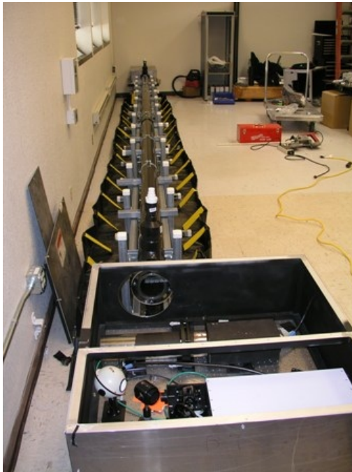
Figure 5–5: Photographs of external water transparency measurement devices at LLNL (horizontal) at left and UCI (vertical) at right.
