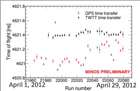
Figure 9. Time of flight between MI60 and Near Detector, using both GPS and fiber TWTT time transfer
