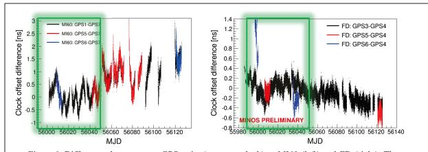
Figure 6. Differences between two GPS units (common clock) at MI60 (left) and FD (right). The green shaded area shows the data used in this analysis. The black points are fixed GPSs and the red and blue the difference between a travelling GPS and a fixed one.
