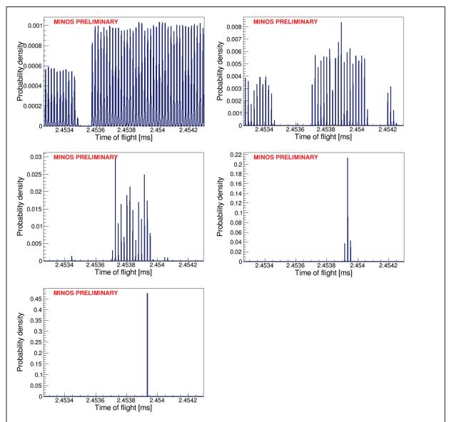
Figure 8. Portion of likelihood function for neutrino time of flight between MI60 and Far Detector for 1 (top left), 10 (top right), 30 (center left), 60 (center right) and 195 (bottom left) events. As we acquire more data, large ranges of time of flight are excluded because of the coarse time structure of the neutrino spill, and each individual peak narrows as the phase of the 53 MHz structure is better measured.
