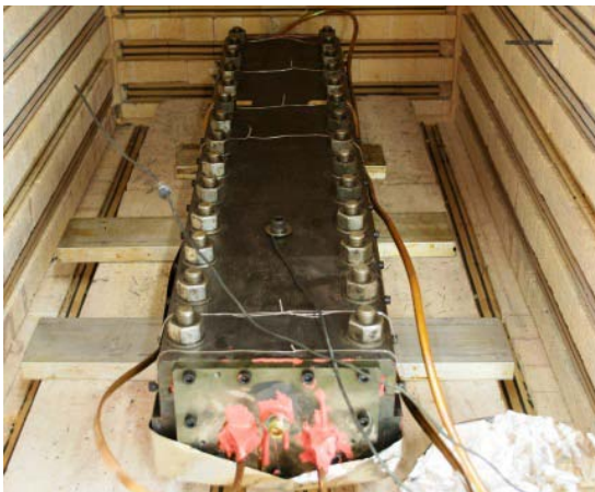
Fig. 4. Coil impregnation fixture in oven.
