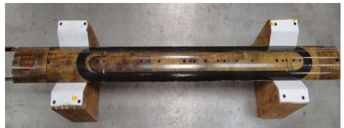
Fig 5. Coil after impregnation with Matrimid 5292.
