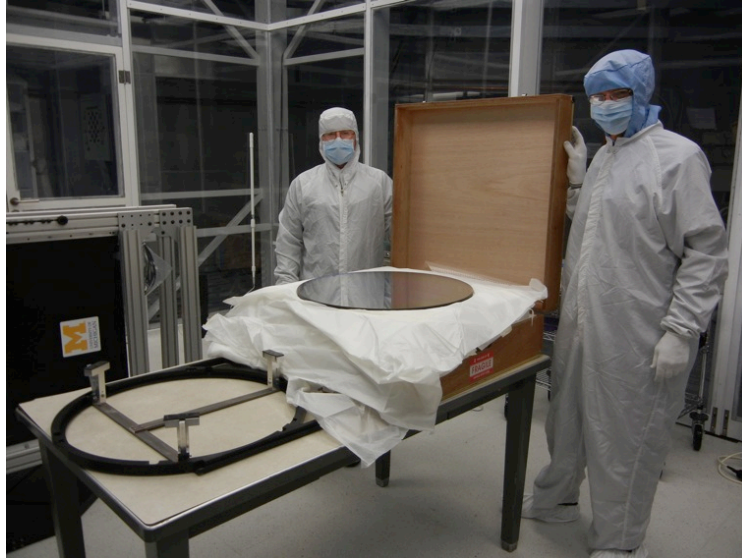
Figure 8 Jan. 2012 DECam filter ready for installation in filter cell in the clean room at CTIO.
