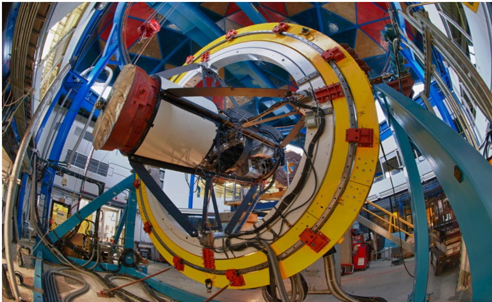
Figure 9. The telescope simulator at Fermilab with DECam installed in Feb. 2011.
