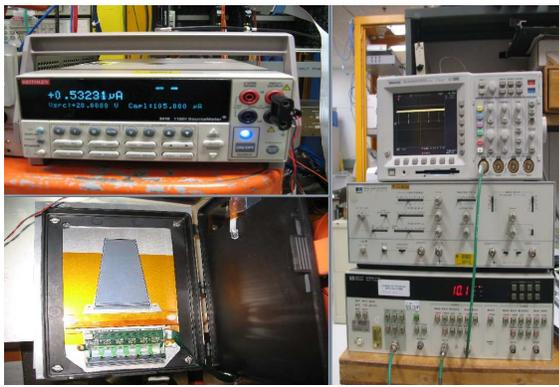
Figure 3. The picture shows part of the SMT test-stand setup: sensor and a light emitting diode (lower left), PS (upper left), optional signal delay generator with respect to the Tevatron clock (right).
