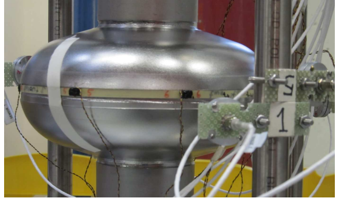
Figure 1: OSTs installed on 1-cell cavity.
