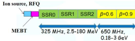
Figure 1: Schematic of the Project X Linac.
