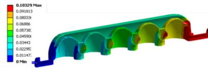
Figure 3: Longitudinal deformation of an elliptical cavity due to 1.0 bar internal pressure (units: mm).
