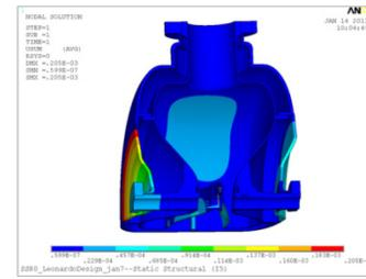
Figure 2: Optimization of the circular rib position of a spoke cavity to minimize  $df/dP$ .
