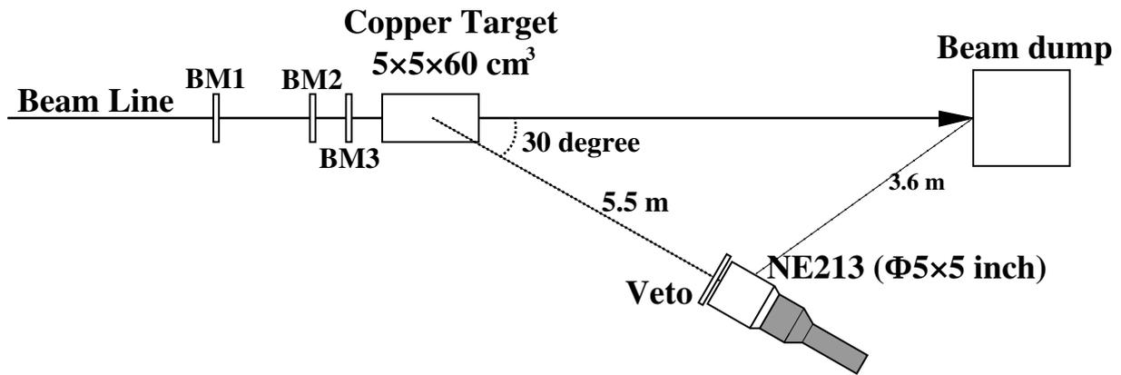
Fig. 1 Schematic view of experimental setup. 120 GeV proton beam comes from left side. Number of protons were counted by three plastic scintillator (BM1,2,3). Copper target, the dimension of which is 5 x 5 x 60 cm, was placed on the beam path. NE213 scintillator with Veto plastic scintillator was placed at 5.5 m from the target, 30° with respect to beam axis.
