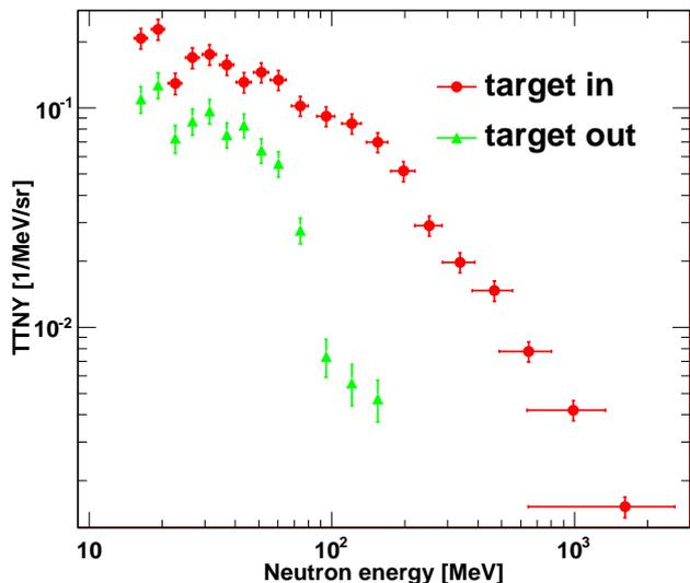
Fig. 4 Double differential neutron yield for 120 GeV proton incidence on 60 cm copper target. The results are compared with results of target out measurement, and include neutrons from floor and dump below 200 MeV.
