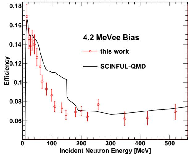
Fig. 3 Experimental and calculated neutron detection efficiencies of the NE213 scintillator at 4.2 MeV bias.
