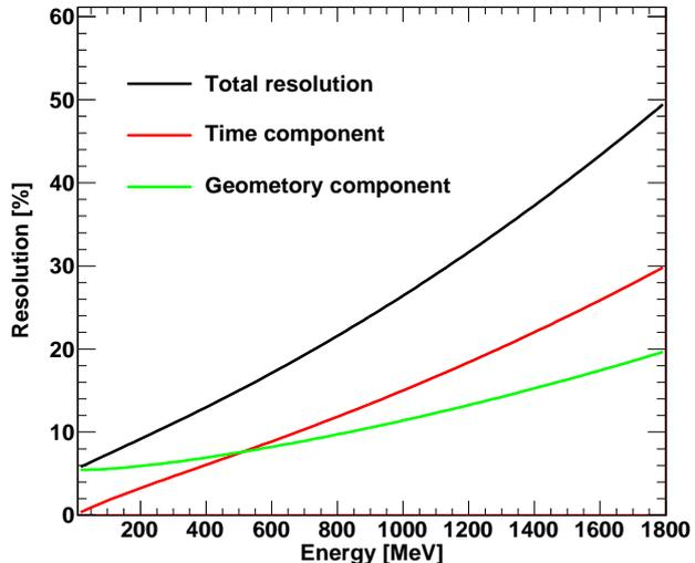
Fig. 5 Energy resolution for TOF measurement. The geometry component depends on thickness of the target and the NE213 scintillator. The time component is derived by full width at half maximum of flash gamma peak.
