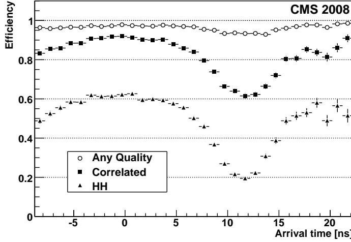
Figure 4: Efficiency of the DT Local Trigger as a function of the muon arrival time in the chamber, defined with respect to the  $t_{\text{Trig}}$  time reference. Results for a chamber of type MB1 are shown as an example, for various types of trigger quality.
