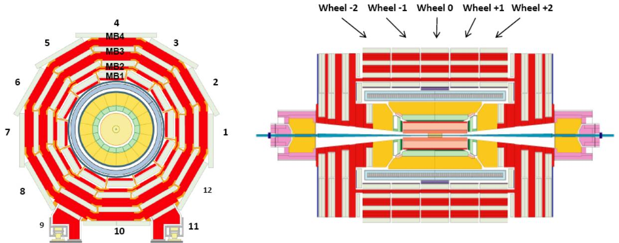
Figure 1: Left: schematic view of one of the five wheels of the muon barrel system of the CMS experiment, in the  $x$ - $y$  plane. Right: the five wheels are visible in the longitudinal view of the CMS detector.
