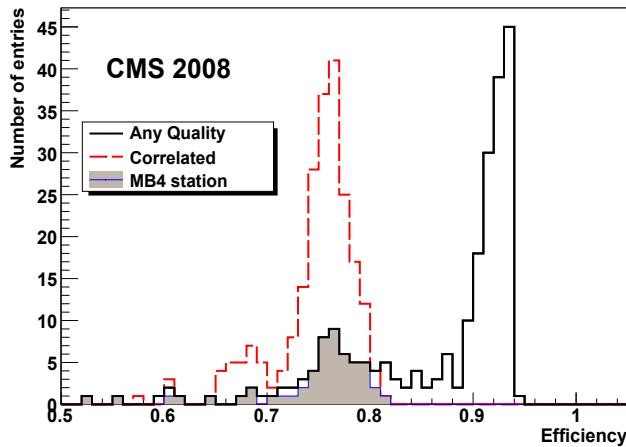
Figure 5: Distribution of the DT Local Trigger efficiency in the  $\phi$  view of the muon chambers, for events selected by the RPC trigger. Each entry corresponds to one barrel chamber. Results for any trigger quality and for correlated triggers are shown. The shaded histogram represents the results for station type MB4, for which only correlated triggers are provided.
