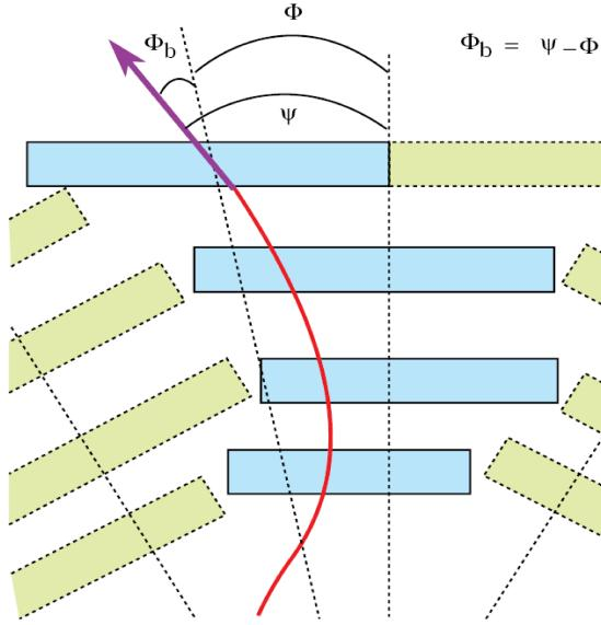
Figure 3: Definition of the  $\Phi$  and  $\Phi_b$  parameters provided by the DT Local Trigger, shown for the outermost muon chamber. The angle  $\psi$  represents the inclination of the trigger segment with respect to the direction perpendicular to the chamber plane. The angle  $\Phi$  is defined with respect to the center of the chamber.
