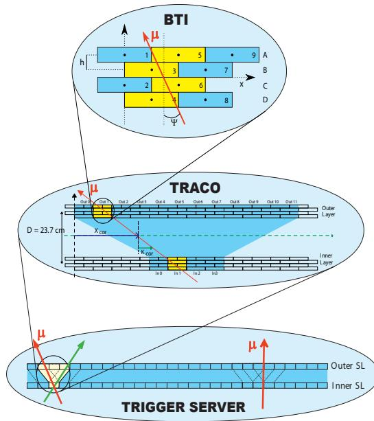
Figure 2: The main components of the DT Local Trigger in the  $\phi$  view of a muon chamber. The BTIs detect hit alignments within each superlayer, the TRACOs search for a proper matching between superlayers, and the Trigger Server selects the best two candidates in the chamber and applies a ghost-suppression algorithm.
