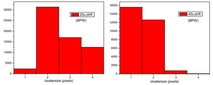
Fig. 14. Cluster size distribution for  $20\ \mu\text{m}$  (left) and  $40\ \mu\text{m}$  (right) pixels applying an  $8\sigma$  seed and  $3\sigma$  neighbor cut.
