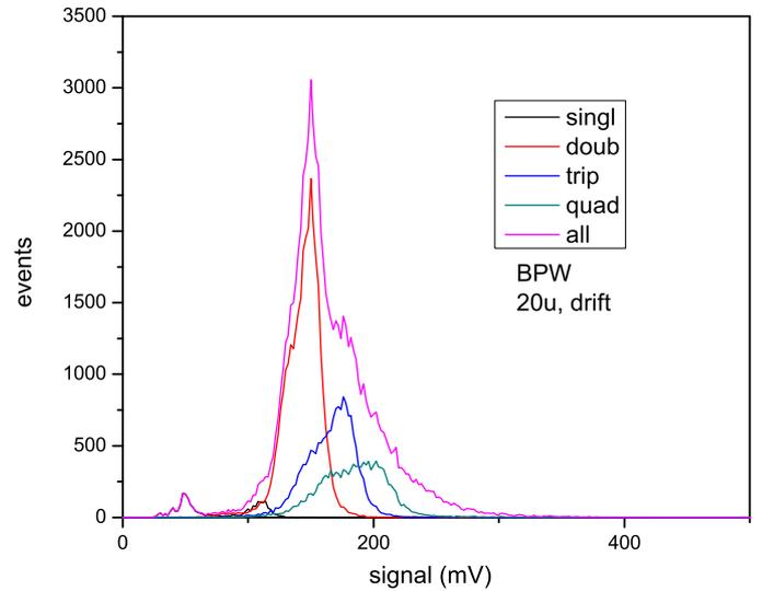
Fig. 15.  $^{55}\text{Fe}$ -spectrum split up into contributions from different cluster sizes (1-4 pixels) as well as the full spectrum.
