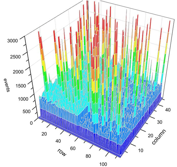
Fig. 11. Flatfield exposure of the 20  $\mu\text{m}$  pixel part using  $^{55}\text{Fe}$  operated in standard depletion with 3 V at the backside.
