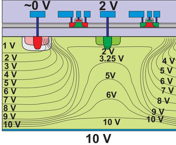
Fig. 2. Illustration of biasing a detector in the drift scheme using 10 V at the backside and 2 V at n-rings on the front side.
