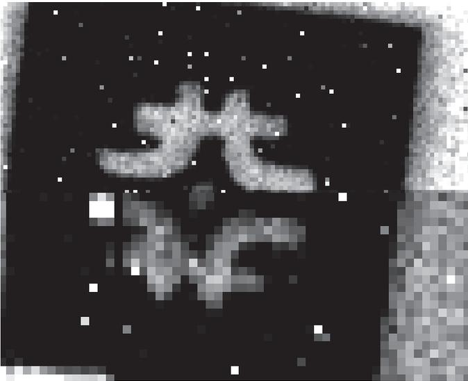
Fig. 10.  $^{55}\text{Fe}$  radiogram obtained with the tungsten logo mask. The grey scale ranges from 0 to 80 hits, indicated by black and white, respectively.
