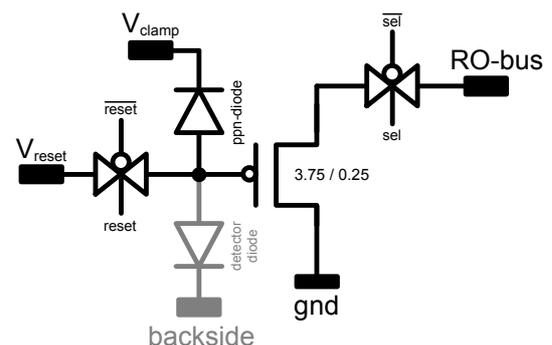
Fig. 6. Pixel schematic following a traditional 3T scheme (source follower, reset and select) with an optional clamping diode to protect the input node.
