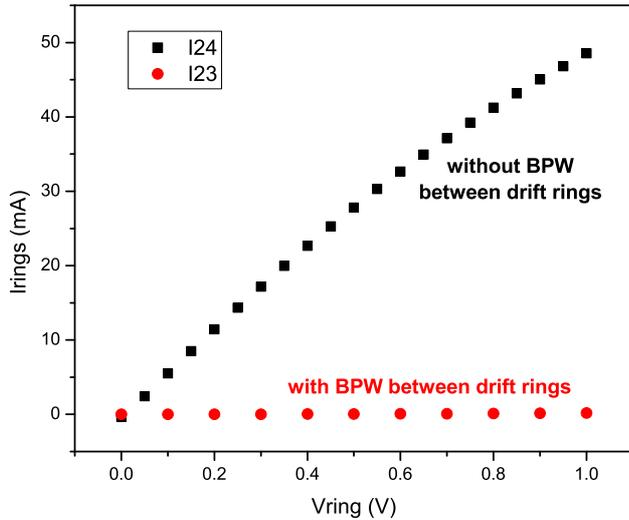
Fig. 8. Cross current (for 322 pixels) between the two drift rings in the  $40\ \mu\text{m}$  pixel, with and without the use of BPW as a p-stop.
