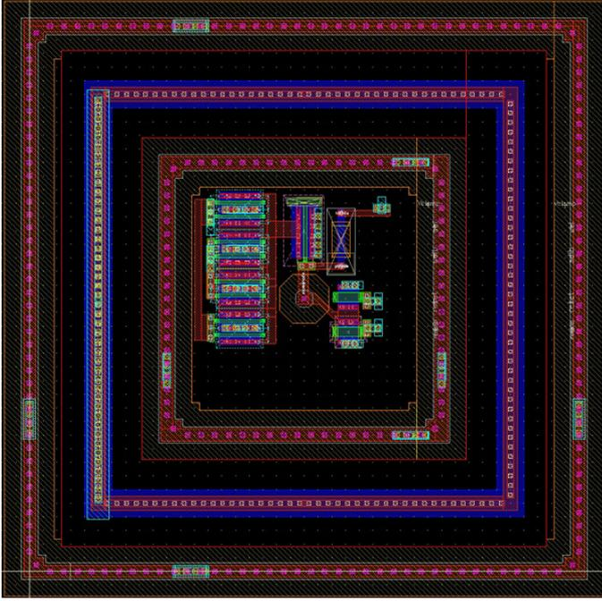
Fig. 7. Layout of the  $40\ \mu\text{m}$  pixel cell with 2 drift rings.
