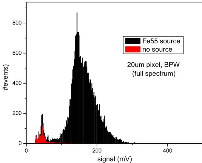
Fig. 13. Full  $^{55}\text{Fe}$ -spectrum for the  $20\ \mu\text{m}$  pixel part.
