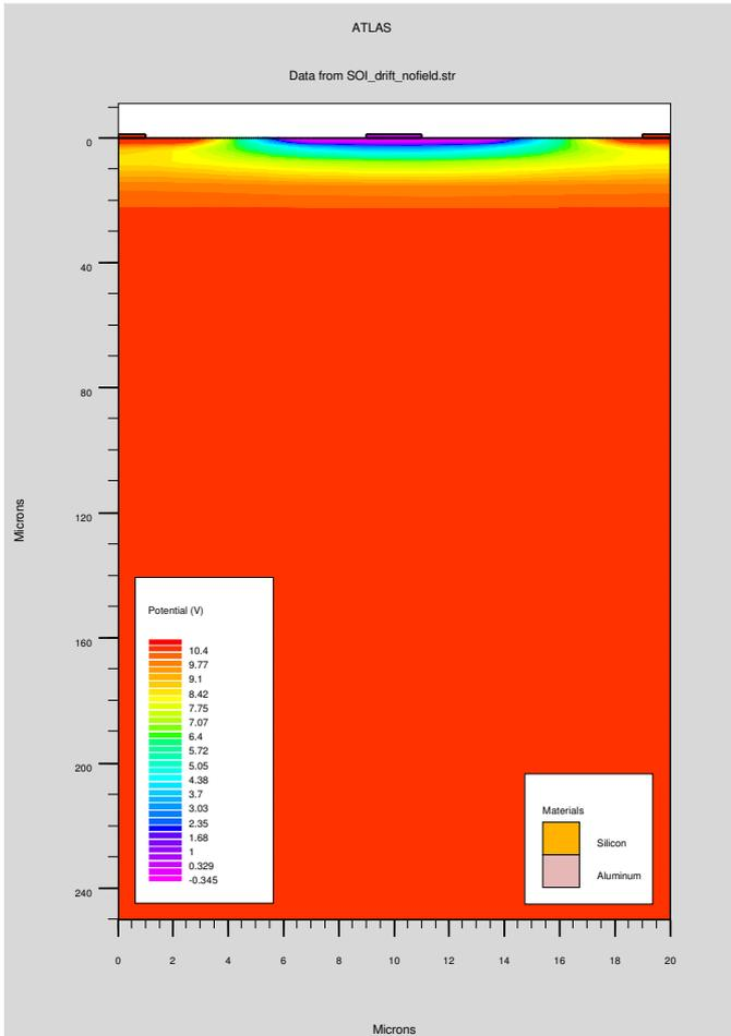
Fig. 4. Silvaco (ATLAS) simulation of a 250  $\mu\text{m}$  thick detector in standard depletion scheme with 10 V at the backside.
