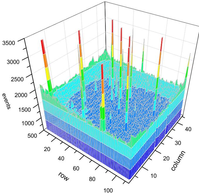
Fig. 12. Flatfield exposure of the 20  $\mu\text{m}$  pixel part using  $^{55}\text{Fe}$  operated in drift scheme with 3 V at the backside and 1.5 V at the n-rings.
