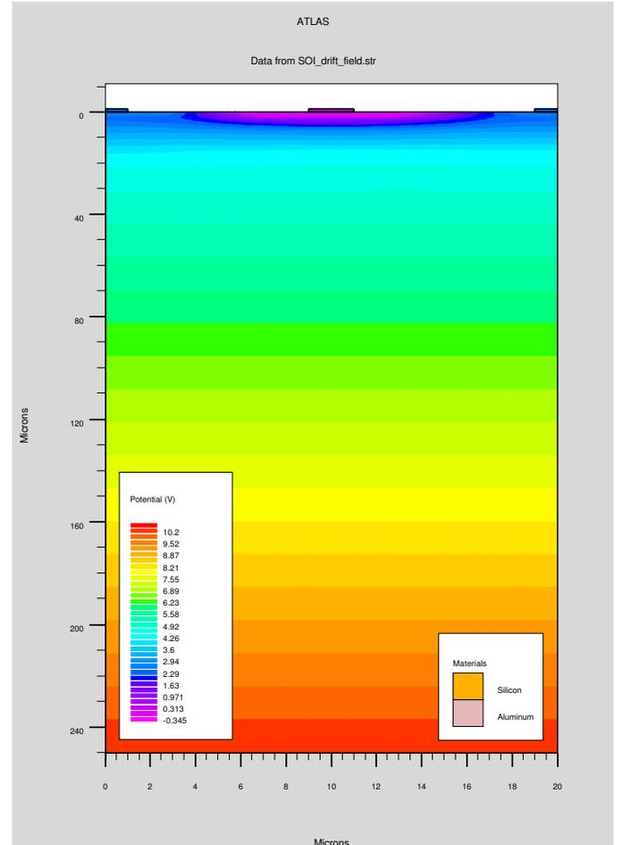
Fig. 3. Silvaco (ATLAS) simulation of a 250  $\mu\text{m}$  thick detector applying drift scheme with 10 V at the backside.
