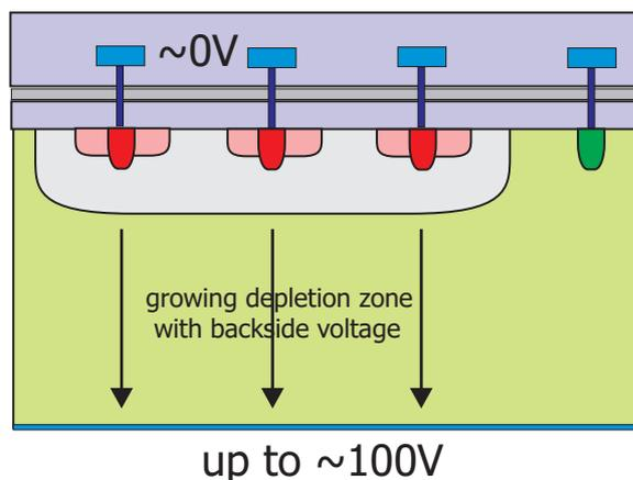
Fig. 1. Illustration of biasing a detector in the standard depletion scheme by applying a voltage at the backside with respect to the potential at the front side diode implantation.
