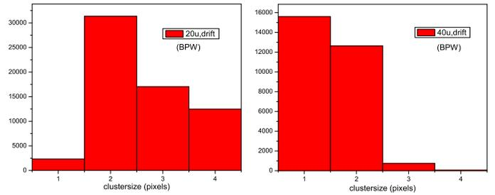
Fig. 14. Cluster size distribution for 20  $\mu\text{m}$  (left) and 40  $\mu\text{m}$  (right) pixels applying an  $8\sigma$  seed and  $3\sigma$  neighbor cut.
