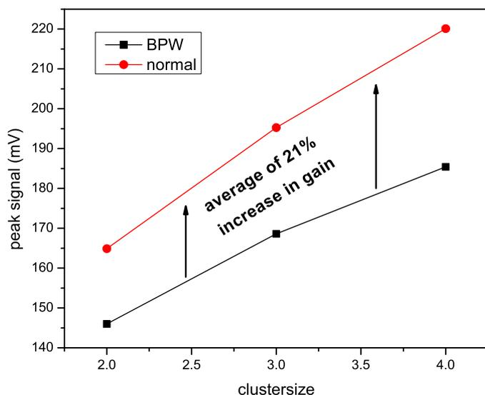
Fig. 16. Comparison of peak energy for p-diode using minimum surrounding BPW and without any BPW (normal).
