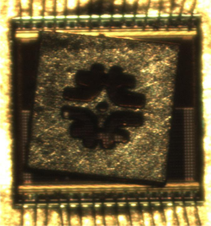
Fig. 9. Micro photograph of the 2.5 mm  $\times$  2.5 mm large chip, a tungsten mask with an engraved Fermilab logo is placed on top.
