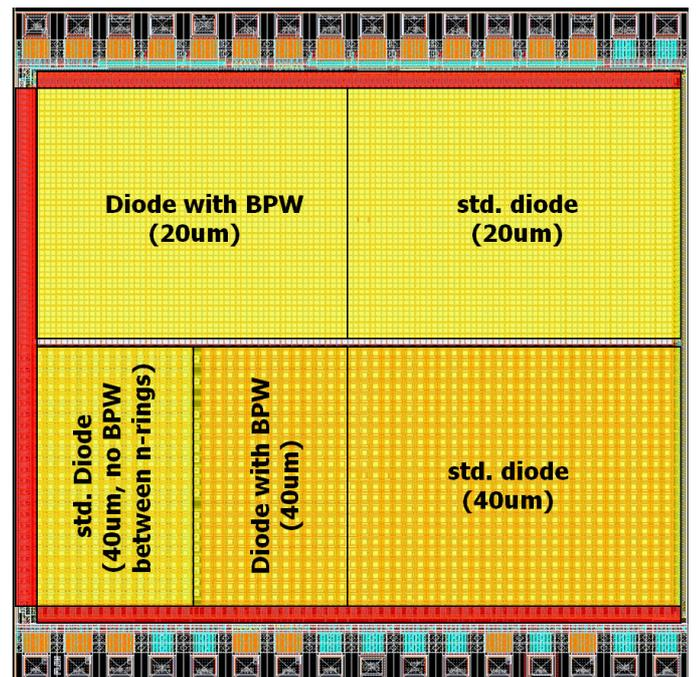
Fig. 5. Overview of the different pixel variations (with and without BPW, 20  $\mu\text{m}$  and 40  $\mu\text{m}$  pixel pitch) realized on the 2.5 mm  $\times$  2.5 mm large chip.
