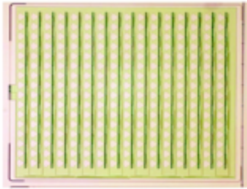
Figure 3: On the left is a MKID demonstration array. On the right is a planar phased array of antennas coupled to detectors. Each of the 64 elements measures both polarizations. Multiple sub arrays may be combined. Both of these examples are from Caltech/JPL.
