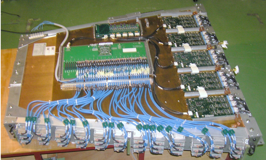
Fig. 4. Assembled ME2/1 chamber showing on-chamber electronics.
