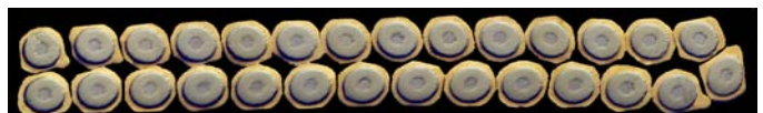
Fig. 5. The Cross-section of a rectangular Rutherford cable made with 27 F4 Nb 3 Al strands, with a high compaction factor of 86.5 %. 13.95 x 1.85 mm 2 .
