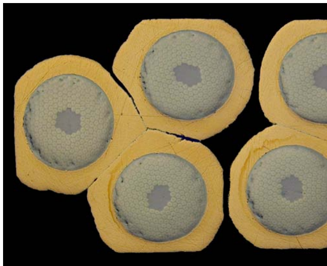
Fig. 6. Expanded cross section of F3 Nb 3 Al strands at the narrow edge of the keystone Rutherford cable, which were used for the SR05 magnet. Copper stabilizer is plastically deformed, but the RHQT precursor is deformed only slightly. No debonding between the outermost Nb layer and the electroplated copper stabilizer is observed.
