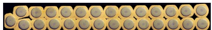
Fig. 4. The cross section of a keystoneed Rutherford cable made with 27 F3 Nb 3 Al strands, with a high compaction factor of 87.0 %.
