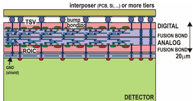
Fig. 9. Cross-section of a 4-side buttable pixel detector tile.
