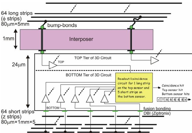
Fig. 5. Block diagram of the prototype unit implementing L1 trigger in the tracker upgrade of the CMS experiment at SLHC using the VICTR chip.
