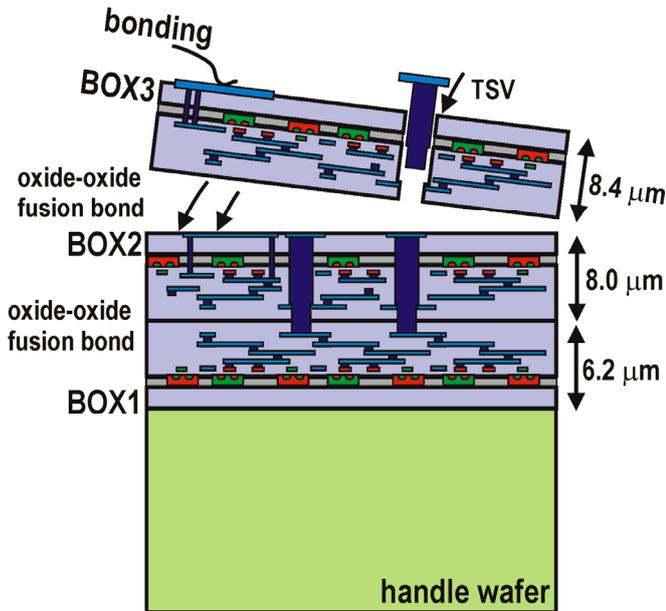
Fig. 1. Conceptual representation of the fabrication of a 3D-IC chip using the via last method and circuits manufactured on CMOS SOI type wafers.
