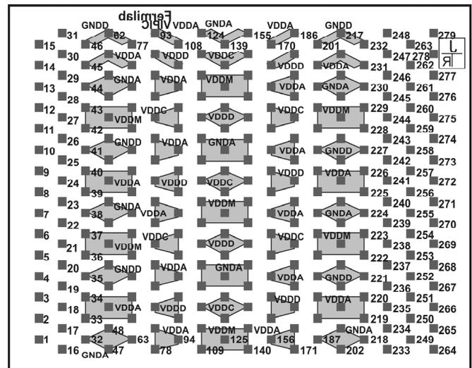
Fig. 8. Back-side view of the chip with bump-bonding pads distributed over the whole surface of the chip; the polygon shadowed shapes mark pins holding the same potential and the same use.
