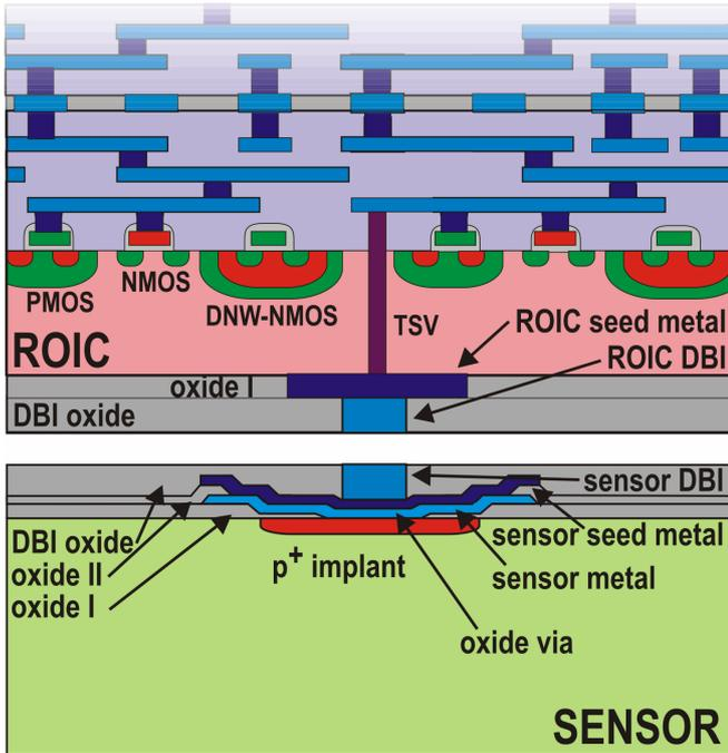
Fig. 10. Cross section of a single fusion bonding node of a 3D readout chip to a detector using the Ziptronix's DBI technology.
