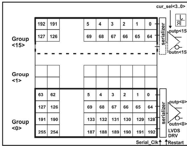
Fig. 6. Block diagram of the VIPIC chip.
