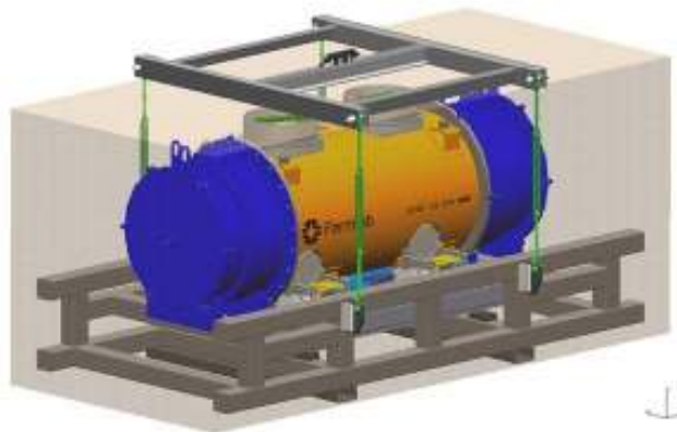
Figure 2: Solid model of cryomodule transport assembly.
