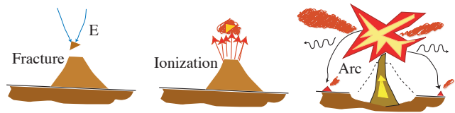
FIG. 1: The three stages in breakdown: fracture, ionization, and arc development.
