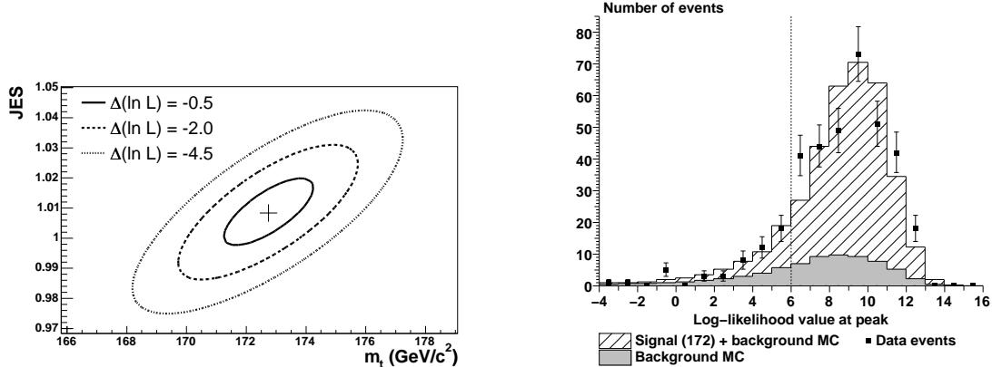
FIG. 15: Left: Measured 2-D likelihood on the data events. The plot shows the contours corresponding to a  $1-\sigma$ ,  $2-\sigma$ , and  $3-\sigma$  uncertainty (assuming Gaussian behavior) in our measurement. The calibration derived from MC events has been applied to both axes. The marker shows the point of maximum likelihood. Right: Likelihood peak position of the individual likelihood curves for data and MC events. The dashed line indicates the likelihood cut of 6 employed.
