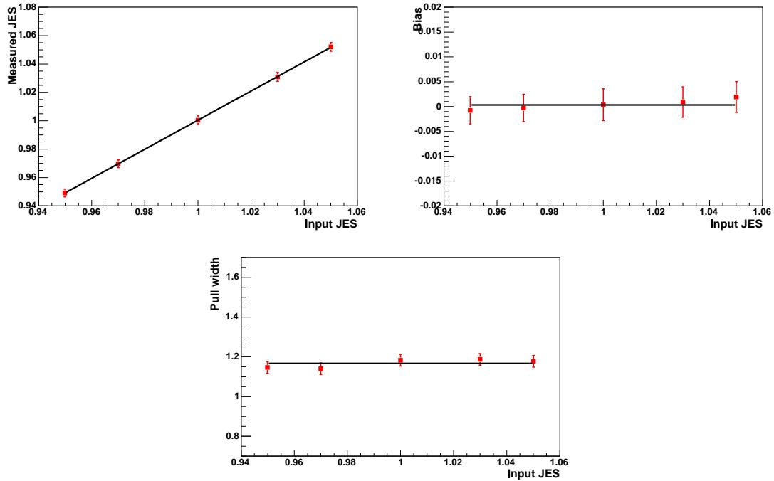
FIG. 13: JES pseudoexperiment results using fully simulated signal and background events after applying a likelihood cut, with a mean of 303 events for each PE. The top quark mass here is fixed at  $m_t = 170 \text{ GeV}/c^2$ . Top left: reconstructed vs. input JES; top right: JES bias vs. input JES; bottom: JES pull width vs. input JES.
