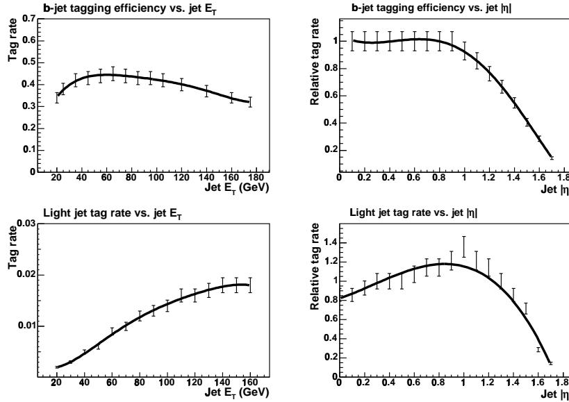
FIG. 4: Efficiency for the SECVTX algorithm. The top two plots show the tag efficiency for tagging  $b$ -jets as a function of the jet  $E_T$  (left) and  $|\eta|$  (right), and the bottom two plots show the tag rate for light jets (mistags), also as a function of jet  $E_T$  (left) and  $|\eta|$  (right). The fits used as a parameterization in our analysis are also shown.
