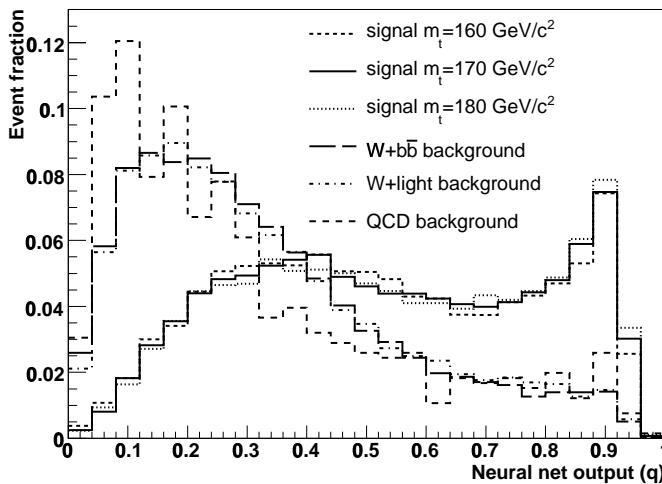
FIG. 10: The distributions of our neural network discriminant variable for signal and background MC events. The peaks on the right are from  $t\bar{t}$  signal events at three top masses. The peaks on the left are from various types of backgrounds.
