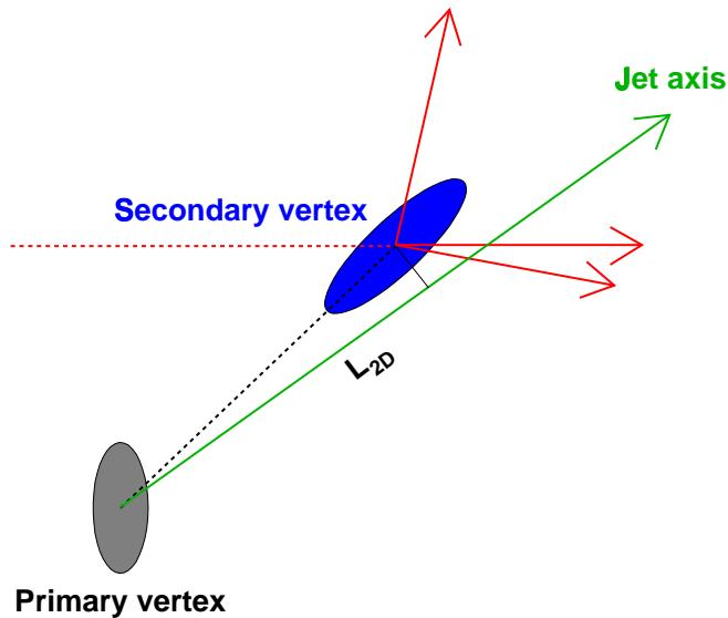
FIG. 1: A view of a  $b$ -jet in the  $x$ - $y$  plane.  $L_{2D}$ , the distance between the primary and secondary vertices projected onto the jet axis, along with its uncertainty, is used to determine whether a jet originates from a heavy flavor quark.
