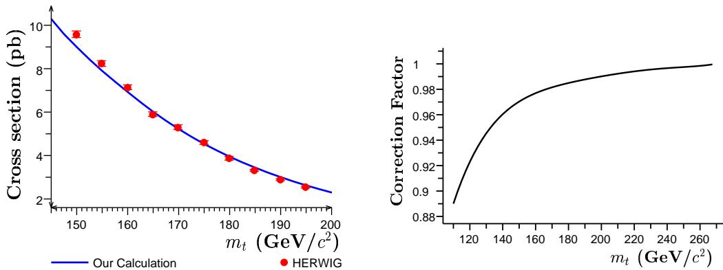
FIG. 8: Left: Cross section obtained from our normalization calculation as a function of  $m_t$  compared with the cross section used in HERWIG. Right: Normalization correction factor due to effective propagators as a function of  $m_t$ .
