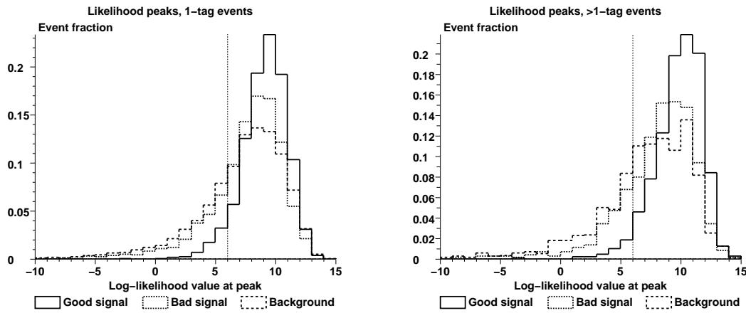
FIG. 11: Distributions of the peak value of the log-likelihood for MC events, divided into “good signal”, “bad signal”, and background events. Left: 1-tag events, right: multiple-tag events. The vertical lines indicate where the likelihood cut is applied.
