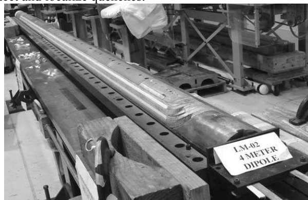
Fig. 1. 4-m long Nb 3 Sn RRP coil.
