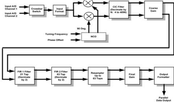
Figure 7: Digital signal processing in the *Graychip* DDC.
