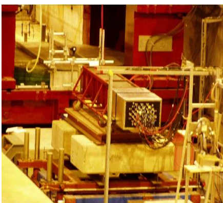
FIGURE 5.45. A DREAM module in the test-beam at CERN. The module is about 2 m in depth and 32 \times 32 \text{ cm}^2 in cross section.
