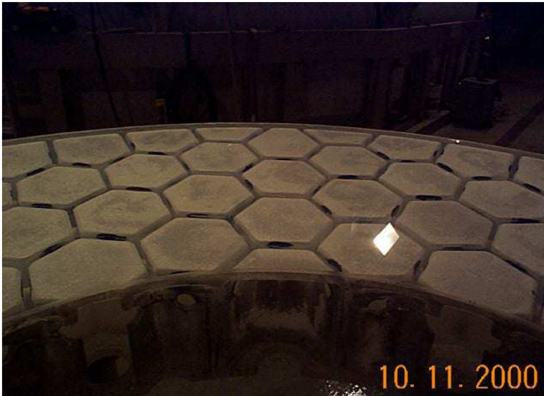
Fig. 7.— Faceplate of the SDSS 2.5 m primary mirror, showing the hexagonal honeycomb structure.
