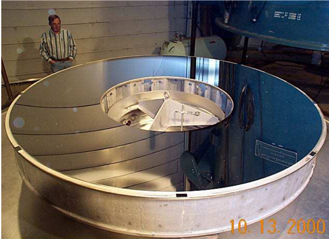
Fig. 8.— SDSS 2.5 m primary mirror immediately after re-aluminizing at the laboratories of Kitt Peak National Observatory, October 13 2000. The first science-grade data were taken after this. The very large central hole is necessary to accomodate the large field, but is even somewhat larger than originally planned (see §6.1).
