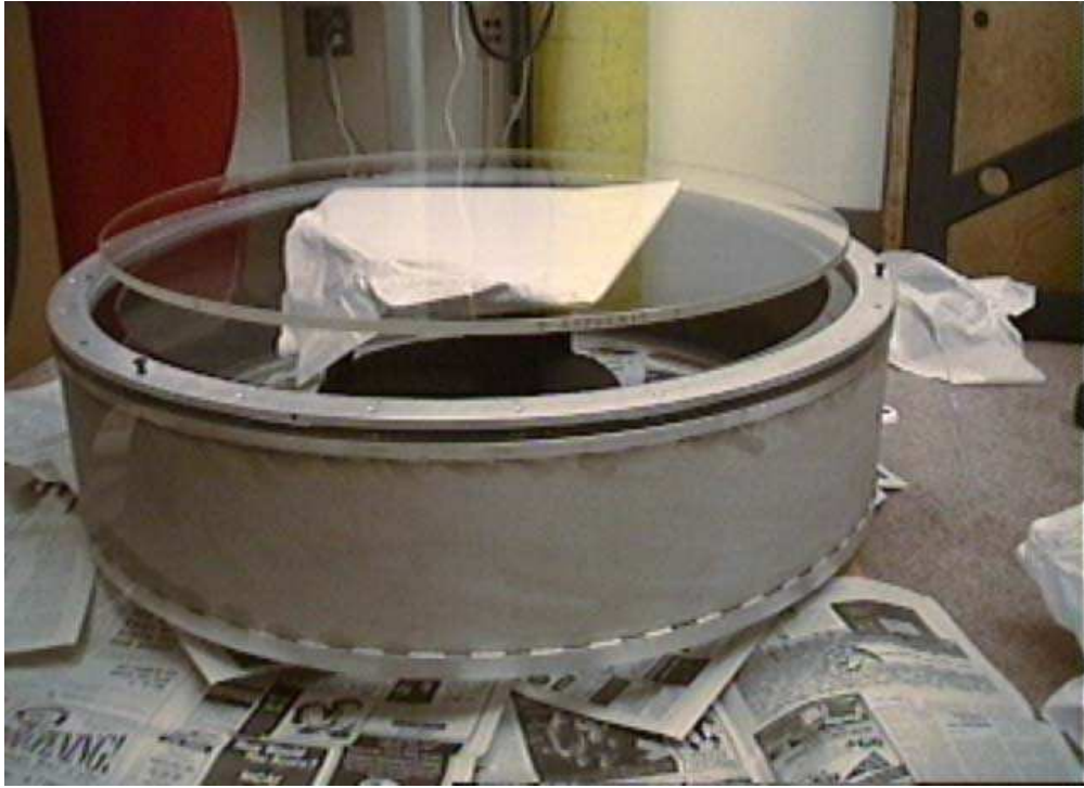
Fig. 10.— The Gascoigne corrector of the SDSS telescope (also known as the “common corrector” because it is used in both imaging and spectroscopic modes) about to be mounted in its cell.
