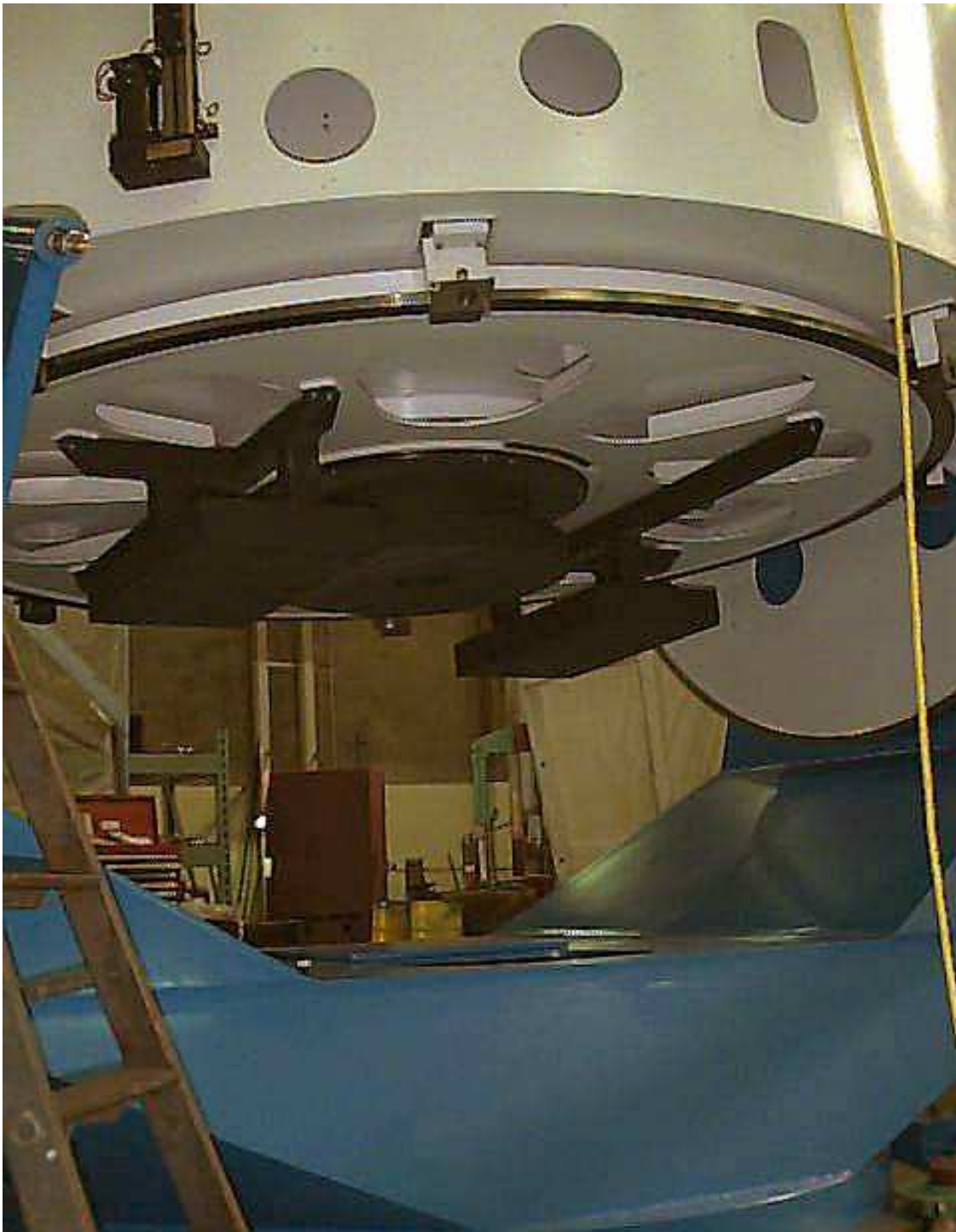
Fig. 26.— Installation of the image rotator on the back of the SDSS telescope, under the primary mirror and covering the rear of the mirror cell. The camera mounts to the central hole during imaging. The spectrographs are permanently mounted on the back of the image rotator (the black mounting fixtures are seen here) and a spectroscopic plug plate replaces the camera in spectroscopic observing mode.
