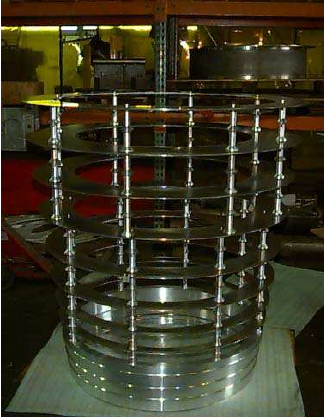
Fig. 19.— The assembled primary baffle (here upside-down in the shop) for the SDSS 2.5 m telescope before painting.
