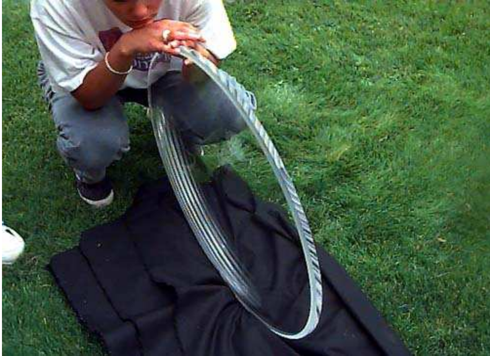
Fig. 11.— Second component of the corrector for the SDSS telescope for use in spectroscopic mode. The strong banding seen is due to multiple internal reflections.
