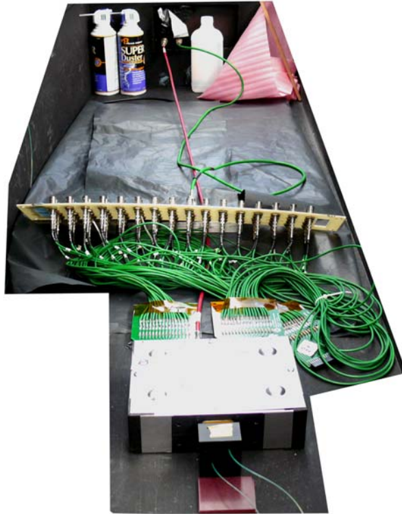
Fig.6. Each MAPMT output was measured independently using this setup.
