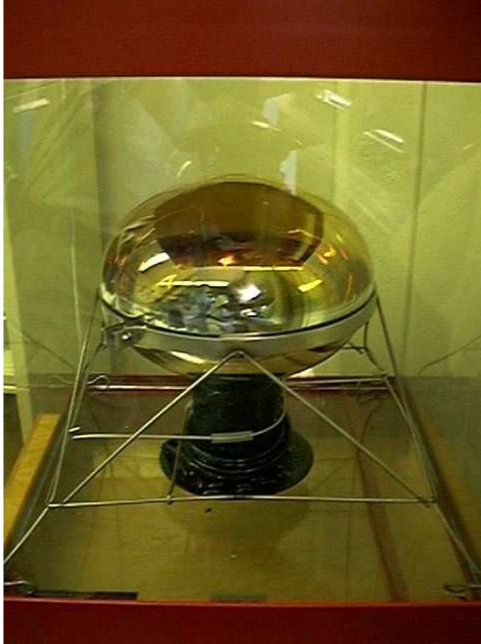
Fig. 1. A typical phototube used in the MiniBooNE detector: an 8 inch R1408 mounted on its wire frame. The base is coated with Masterbond (as described in section 2.1) before the PMT is installed into the detector.
