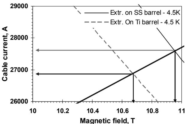
Fig. 8. SR03 short sample limits at 4.5 K.
