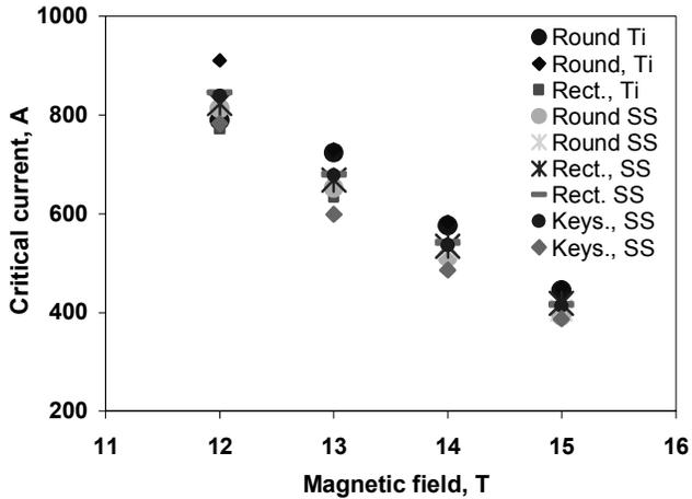
Fig. 4.  $I_c$  at high fields obtained through V-I measurements as a function of magnetic field for 1 mm 108/127 RRP round strands and strands extracted from cables. Ti and SS in legend represent test barrel material.
