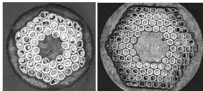
Fig. 1. 54/61 (left), and 108/127 restack (right) RRP designs.
