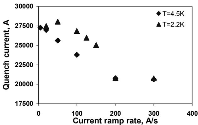
Fig. 7. SR03 ramp rate dependence at 4.5 and 2.2 K.
