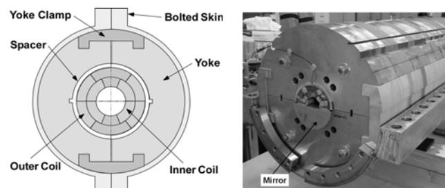
Fig. 1. HFDA dipole and HFDM mirror models with bolted skin.
