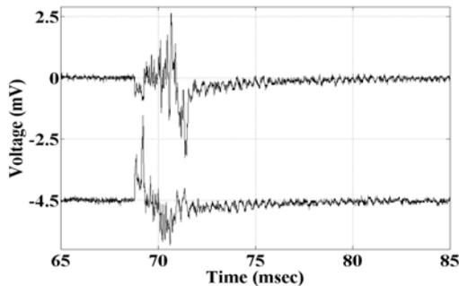
Fig. 7. Superimposition of 'Transport Current' and 'Magnetization' Voltage Spike in sample C
