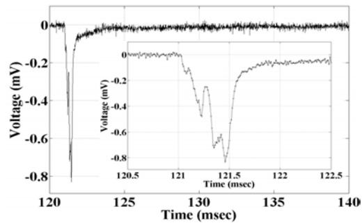
Fig. 9. 'Magnetization' Voltage Spike in sample A – bucked signal
