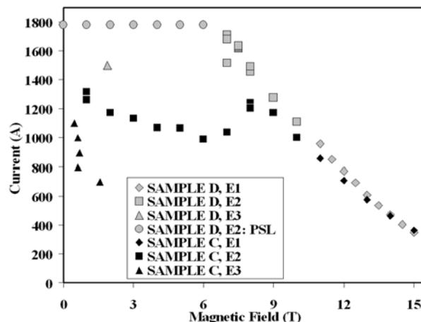
Fig. 2. Critical and quench current of the samples C and D
