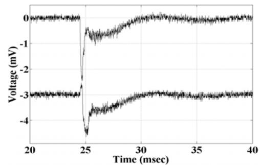
Fig. 3. ‘Magnetization’ Voltage Spike in sample D
