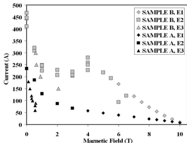
Fig. 1. Critical and quench current of the samples A and B
