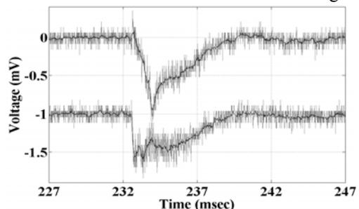
Fig. 4. ‘Magnetization’ Voltage Spike in sample D
