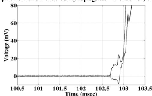
Fig. 8. Voltage spike triggering a quench in sample C
