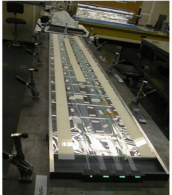
Fig. 7. Assembly of one CPR module: All 54 tiles are wrapped in aluminized mylar foil and the fibers routed to the four output connectors.
