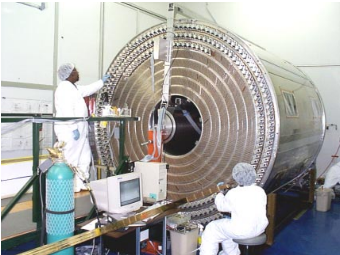
Figure 4. The COT during “stringing” of the wire planes and field sheets. The carbon composite inner cylinder, aluminum end plate (east) and aluminum outer cylinder are visible. Superlayers 1-5 have been strung and superlayer 6 is about half done. A wire plane is being inserted at 10:00 and a field plane at 4:00. Pre-tension fixtures are seen in superlayers 6 – 8.
