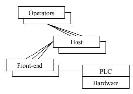
The diagram illustrates multiple links between operators, host computers (VAX) and the front-end computers. Each PLC is connected to a single front-end computer and specific set of hardware elements. The control and monitor of LCW is distributed over a wide range of localities, from the main control room to the field operation.
