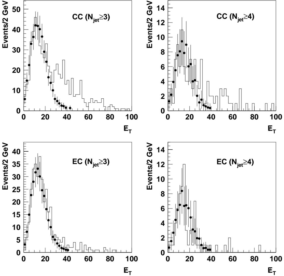
FIG. 4.  $\cancel{E}_T$  spectra of sample 2 (points) normalized to sample 1 (histograms) in the region of  $0 \leq \cancel{E}_T \leq 14$  GeV. The normalizations are done for the fake electron in the CC and EC, respectively. The errors are statistical only.
