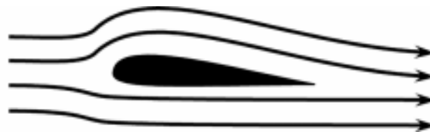
Fig. 2. The Bernoulli description's view of airflow around a wing.
