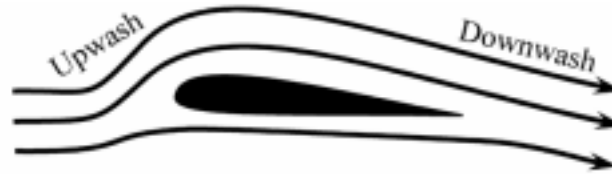
Fig. 3. The true airflow around a wing with lift.
