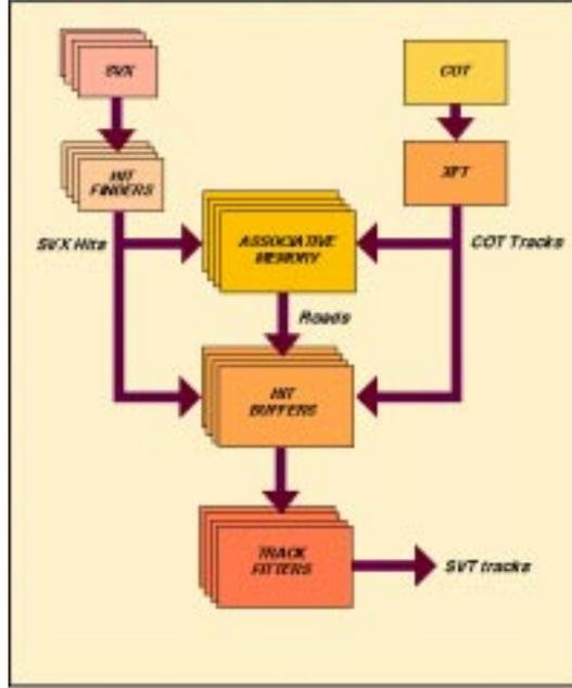
Fig. 1. The CDF Online Silicon Vertex Tracker architecture.
