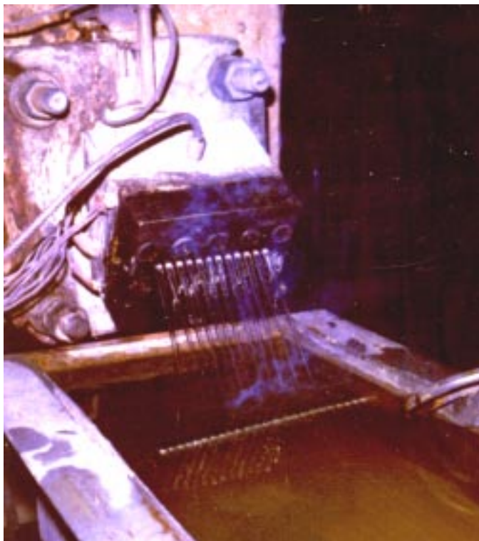
Fig. 2. View of the extruder head showing strings of scintillator.
