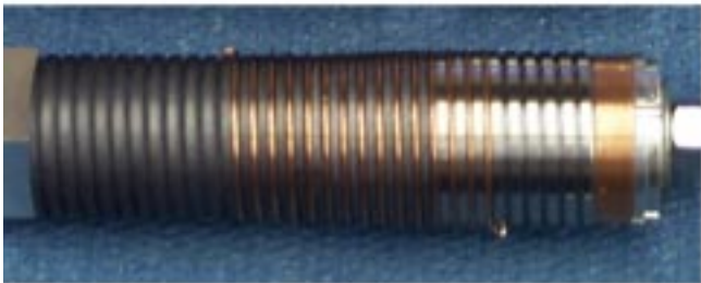
Fig. 2. Photograph of reaction (left) and measurement (right) sample holders during displacement of a sample.
