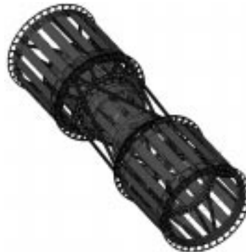
Figure 1. The ISL detector. Only half of the sensors are displayed.
