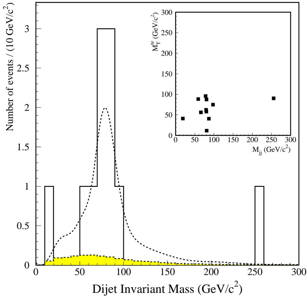
Figure 4: Dijet mass spectrum of the two untagged jets in double  $b$ -tagged events. The shaded curve shows the expected distribution from QCD  $W + \text{jets}$  background and the dashed curve is from  $t\bar{t}$  plus background. The inset compares the lepton- $\cancel{E}_T$ (neutrino) transverse mass to the dijet invariant mass in these eleven events showing evidence for events with both a leptonically-decaying  $W$  and a hadronically-decaying  $W$ .
