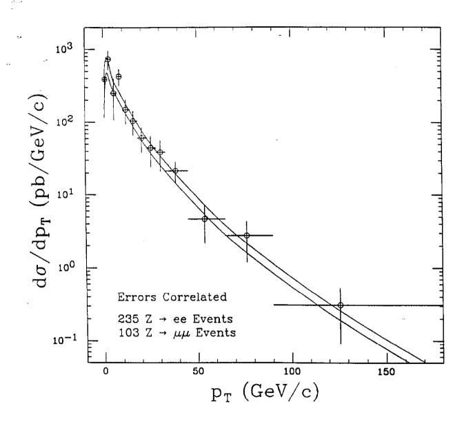
Figure 2: The differential cross-section for Z production. The next-to-leading order QCD calculation is shown as a band; the width of the band indicates the theoretical uncertainty.
