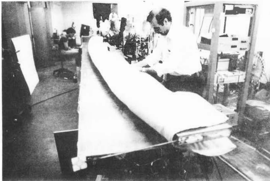
John Satti wrapping a prototype Accumulator vacuum-chamber section for brakeout tests. (Photograph by Fermilab Photo Unit)
