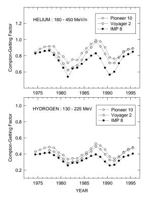
distance with secondary maxima and minima associated Fig.1 Comptonn-Getting factor calculated from with the time of minimum and maximum solar activity in spectra for galactic He and H. cycles 20, 21 and 22. The radial dependence of  $K_{rr}$  for 175
