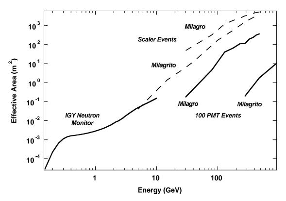
Figure 1 : Effective area curves for Milagro and Milagrito, with an IGY neutron monitor for comparison. (Milagro shower trigger presently requires ≈150 PMTs )
