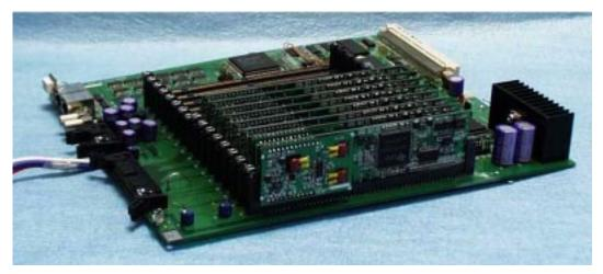
Figure 4: Photograph of the prototype signal finder module. The height of the module is 6U but the depth of the module was extended to 26 cm.
