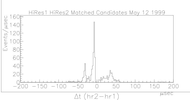
Figure1: Time difference for matched events from the HiRes1 and HiRes2 detectors. The peaks correspond to tracks produced by vertical flashers located at various positions between the 2 detector sites.
