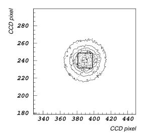
Figure 2: A CCD image of Canopus on the optic axis. The axes are in unit of CCD pixels, corresponding to a  $6.7 \times 10^{-3}$  degree pitch. z axis is in arbitrary unit. A square overdrawn is a scale of a pitch of the camera (0°.12 square).
