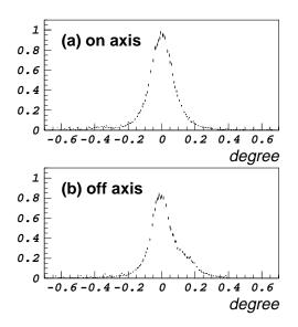
Figure 3: Measured radial point spread functions on the optic axis (a) and 1°.25 off the axis (b) are shown in a unit of degree. The zeros of the abscissa are arbitrary, and vertical scales are normalized by the peak height of (a).
