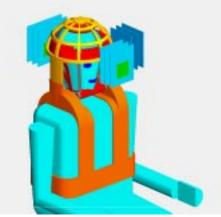
The detector system is constituted by a mechanical structure devoted to interface an helmet, three silicon detectors, the EEG and the stimulator. The silicon detectors will be positioned in front of the astronauts eye, in the temporal region and over the occipital region.
