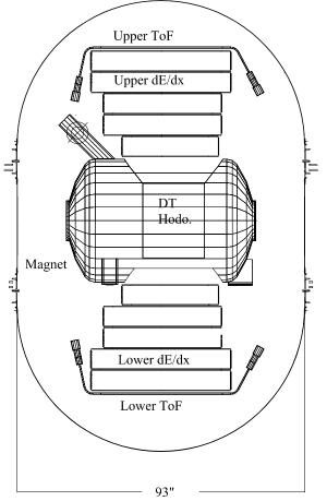
Figure 2: Cross-section drawing of the HEAT magnet specin the magnet dewar.
