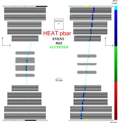
tamination. Based on the HEAT data, Figure 3: Orthogonal views of a sea-level muon passing through the HEAT-pbar we find that the combined negatively instrument with the 1T (central field) magnet on.
