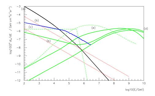
Figure 1: Comparison between different sources for neutrino induced muons: (a) atmospheric induced muons, (b) interactions with the interstellar medium (upper curve for  $l = 0^{\circ}$ ,  $b = 0^{\circ}$ , lower curve for  $b = 90^{\circ}$ ) (Domokos 1993) (c) this calculation (d) AGN jet models: (Mannheim 1995) and (Protheroe 1996), (e: dashed dotted) AGN disk models: (Nellen et al. 1993) left and (Stecker 1993) right.
